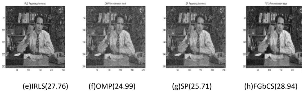
Fig.4 Noisy video reconstructed results in terms of PSNR in frame 20
