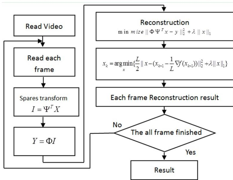
Fig 1 The processing of noisy video compressive sensing
